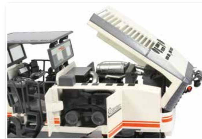
Opening engine cover and side doors.
