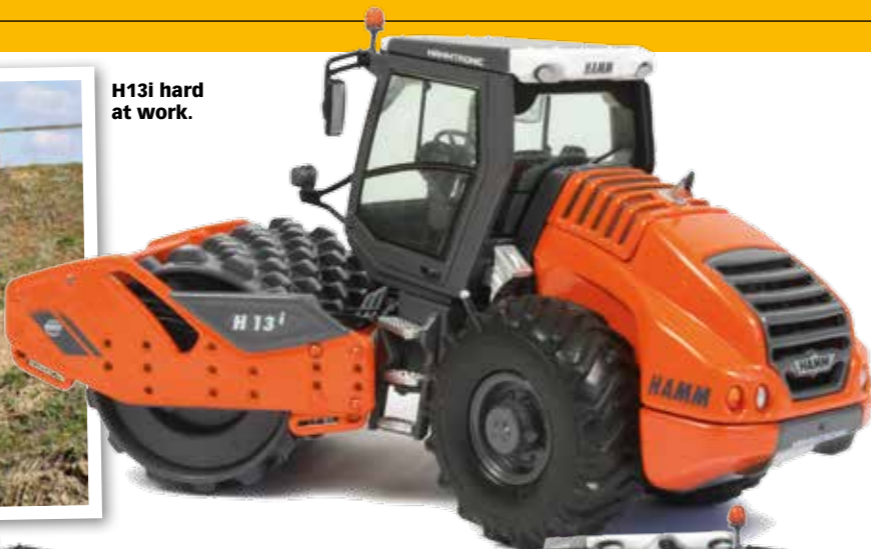
Above and right: Hamm H13i pad foot drum.
